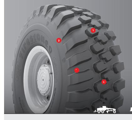
The VersaBuilt All Traction radial tire is designed to provide serious traction, dependable performance, and versatility in loader and grader applications.
