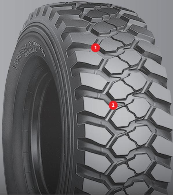
The V-Steel F-Traction (VFT) radial tire for haulage applications.
