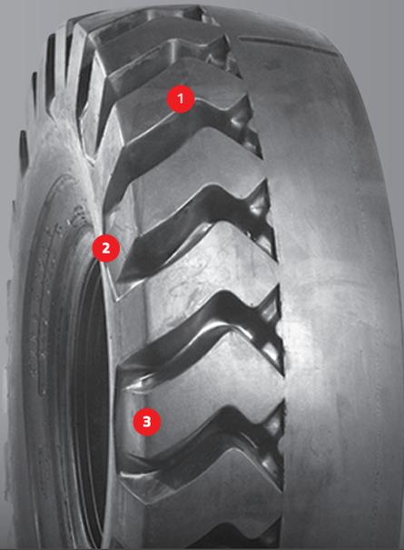
The Half Tread Loader Dozer (HTLD) bias tire is specifically designed for loader applications including giant loaders in mining operations. Provides excellent traction with half deep lug tread design and outside shoulder protection.
