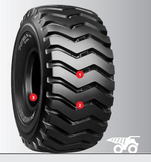
The V-Steel R-Lug (VRL) Premium radial tire is designed for earthmover and scraper applications, and features good traction and excellent cut resistance.
